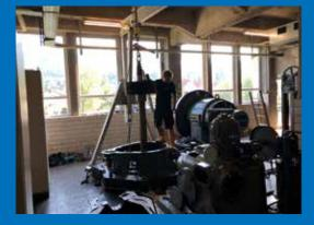
Manoeuvring an old gearbox and generator out of a 1950s hydroelectric plant and bringing in a new Permanent Magnet generator called for an innovative transport and handling solution.
