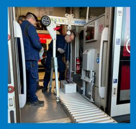
PORTAGANTRY \*\* to DB Group who needed to lift and move large batteries within train carriages. The solution to the tight area of use was to use smaller A-Frames, allowing for safe and easy lifting within the confined area.
