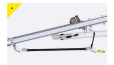
Use the suitable straps to connect on to each shackle point on the gantry, this should form a 'V'.
