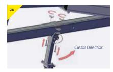
Dring the wheel assembly to the strut and fit them as close to the top of the trap plate as possible. Use the bolts and wingnuts that are provided to secure the assembly aid to the legs. Make sure that it is fitted in the correct orientation so that it allows for the wheel assembly to fold down when not in use.
