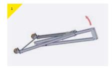
Raise the Porta Gantry A-Frame off of the ground, by approximately 500mm.
