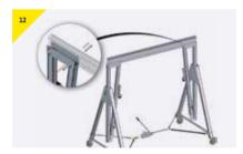
Secure A-Frame A to the beam by placing the bolt provided with the A-Frame.
