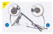
Put the brake on A-Frame A and take off the brake on A-frame B.
