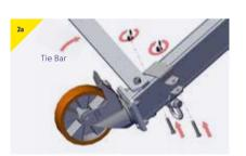
Bring the shackle assembly to the leg whilst facing them inwards, fit them as close as possible to the tie bar. Use the bolts and wingnuts provided to secure the assembly aid to the legs (one in each leg).
