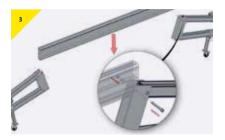
Place the beam on the A-Frames as per the usual gantry assembly (Refer to Gantry Assembly and Operations Guide).
