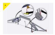
Connect all the straps to the pulling device, locate the pulling device around the centre of the beam. The image above is showing a Tirfor, a chain block can also be used in this instance.
