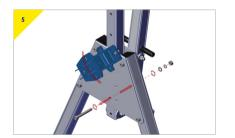
Remove the bottom bolt from the trap plate, and swing the bracket into position.
