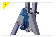
Re-assemble the bracket to the plate. Make sure all the bolts for the bottom connector have been tightened.
