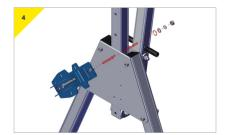
Present the bracket to the trap plate, insert and secure the M16 top bolt supplied with the bracket.
