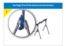
Prepare the bracket to recieve the device, making sure all the bolts for the bottom connector have been tightened.
