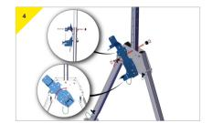
Remove the top bolt whilst holding the bracket on an angle.
