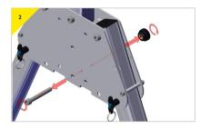
Remove the bottom bolt from the trap plate.
