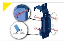
Adjust the width of the wings to 3" (76.2mm) to fit on the T davit column section.
