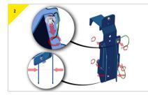
Adjust the width of the wings to 2 1/2" (76.2mm) and fit the bracket onto the Porta Davit Quantum backstay.
