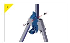
> Insert the supplied M12 top bolt and secure.
