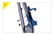
Insert the pins provided with the bracket.
