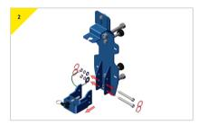
Before attaching the bracket to the device, dissemble the bracket by removing the bottom connector.
