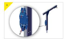
Prepare the bracket to recieve the device and remove the bolt from the bottom connector and loosen the top connector.
