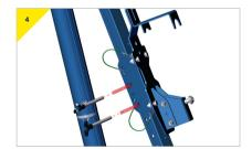
> Insert the pins provided through the bracket.
