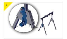
Prepare the bracket to recieve the device, make sure all the bolts for the bottom connector have been tightened.
