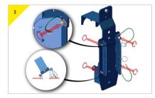
> Adjust the width of the wings to 2" (50.8mm) to fit on the Porta Davit 500 backstay.
