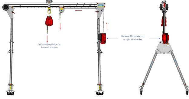
\*Set up is indicative - Various winch brackets available Masterlink or Close Coupled trolley options available.
