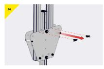
While in this vertical position remove ball lock pin from its stow hole
