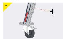
> The foot option can be changed by removing the ball lock pin and withdrawing the foot cartridge
