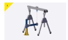
Position the PORTAGANTRY RAMDET over the test davit ensuring the trolley sits directly above the shackle on the beam.
