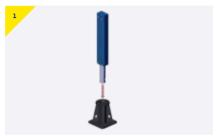
Insert the column into the socket.
