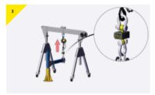
> Ensuring the loadcell reads 0 before starting. Apply load to the test davit using the chain block. Once the required loading has been achieved hold the load for the amount of time determined by the local authority regulations. De-load the test davit by reversing the chain block.
