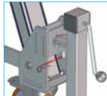
Fig.2 Jacks secured with locking pins and clips
