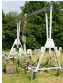
Fig.3 Wind Up Jack Leg system in place – normally used with pneumatic "All Terrain Castors".
