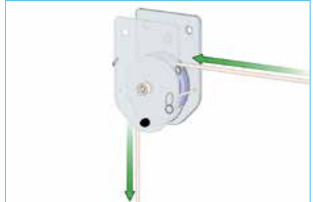
20. Thread Winch Wire/Rope around Sheave on the Sheave Carrier
