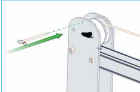
19. Secure Winch Wire/Rope with push pin provided
