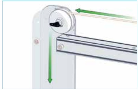
18. Thread Winch Wire/Rope around Sheave
