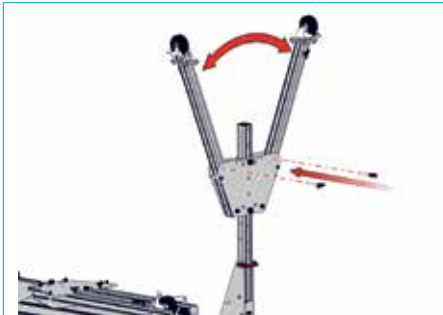
15. Open leg and insert ball-lock pin into second hole securing the leg in its open position. Repeat for second leg.
