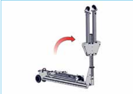
13. Rotate upper Upright to vertical position.
