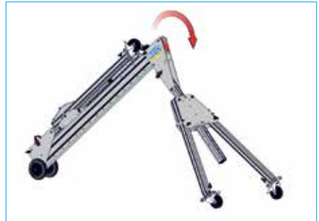
16. Rotate upper Upright around until ball-lock pin is adjacent to beam. Remove pin and continue motion until stops engage beam and holes are aligned, as in steps 6 and 7.
