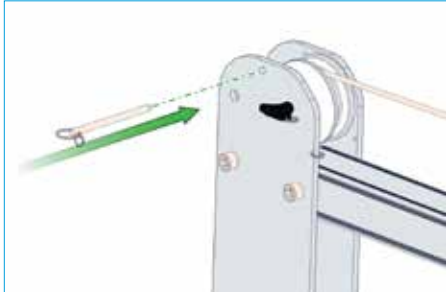
19. Secure Winch Wire/Rope with push pin provided
