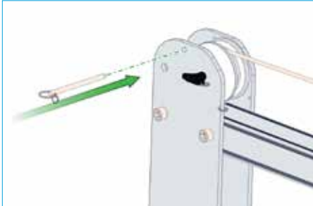
19. Secure Winch Wire/Rope with push pin provided
