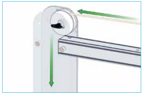
18. Thread Winch Wire/Rope around Sheave
